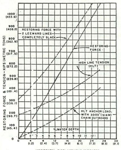
Figure 17 Mooring Analysis - 200 foot water depth
