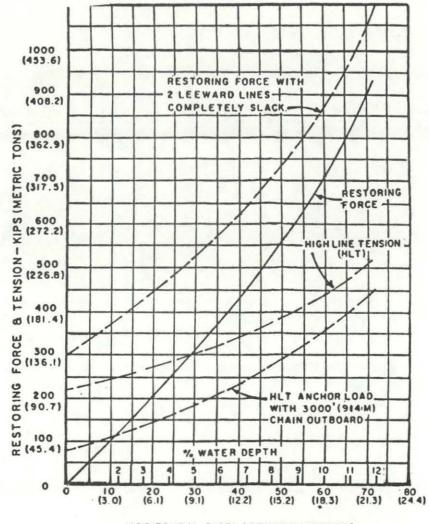
Figure 19 Mooring Analysis - 600 foot water depth
