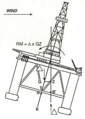
called the metacenter, M. At these small angles a right triangle, G-Z-M, is formed. Because of this triangle, GZ can be expressed trigonometrically in terms of the vertical distance between G and M, and the angle of inclination,  $\Theta$ .
