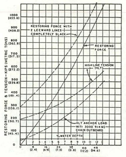
Figure 18 Mooring Analysis - 400 foot water depth
